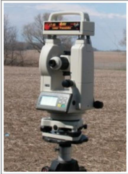
The LT-10 comes with a vertical laser enhancement that allows the instrument to be operated by a single user. Operation of instrument is the same as a normal theodolite and time should be taken to read the manual before use.
